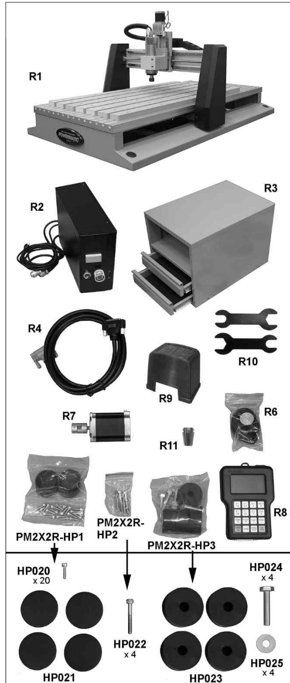
Figure 7-7: PM-2x4SP table contents (not to scale)
