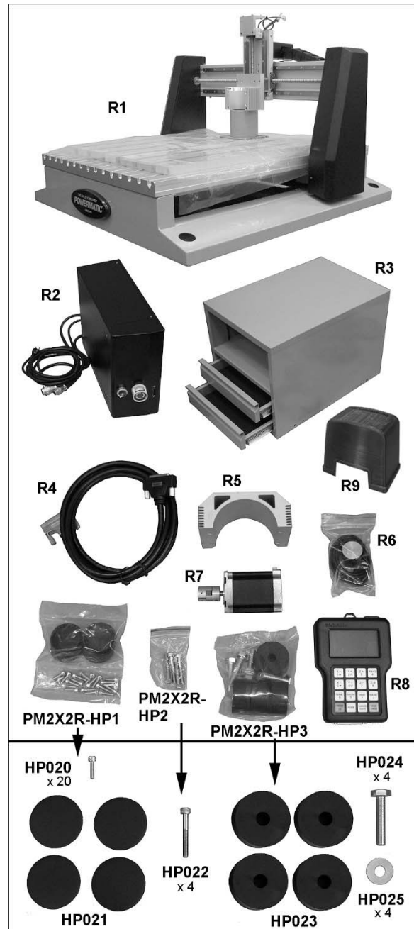
Figure 7-3: PM-2x2R table contents (not to scale)
